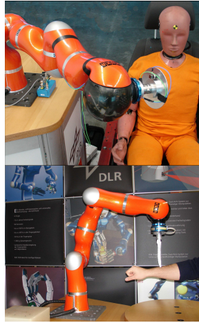
Fig. 3. Collision experiments with an LWR-III, HIII dummy (upper) and human (lower)
