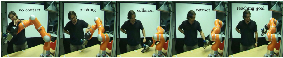
Fig. 6. Automatic recovery from physical collisions with real-time motion planning
