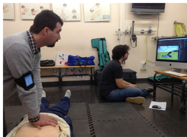
Fig. 6. Experiment of CPR-chest compression on manikin and obtaining the chest compression data from LISSA, iCPR and Lateral PC Skillreporting System
