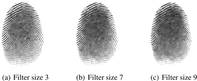
Fig. 2. Examples for the Median Cut Filtering test, applied to an image from DB1 (ID 91_2)
