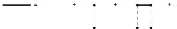
Fig. 4 Bound Coulomb propagator ( double line ) expansion in terms of the free propagator ( single line ). The dashed line corresponds to the Coulomb interaction with the nucleus
