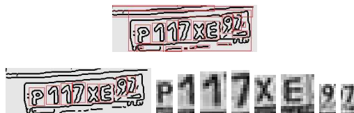
Fig. 3. Symbols envelope determination: envelope determination, non-relevant candidates elimination, symbols segmentation
