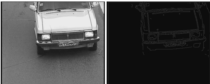
Fig. 4. Canny edge detection over low contrast and deformed vehicle plate
