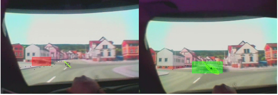
Fig. 5. A car appears on the left of the driving scene and is about to cut the driver’s way. The red bounding box around the approaching hazard and the driver’s fixation cluster are shown. Once the bounding box is intersected by the fixation cluster, the traffic hazard is marked as “perceived”, highlighted by the green bounding box.
