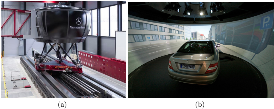
Fig. 3. Moving base driving simulator. The entire cabin is mounted on a hexapod, moving along the 12m rail resulting in up to 1g acceleration force 2 .
