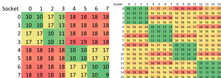
Fig. 2. Distance matrix of the HP (left) and the BCS system (right). The matrix is scaled such that the upper left value is always ten, larger numbers indicate higher distances.
