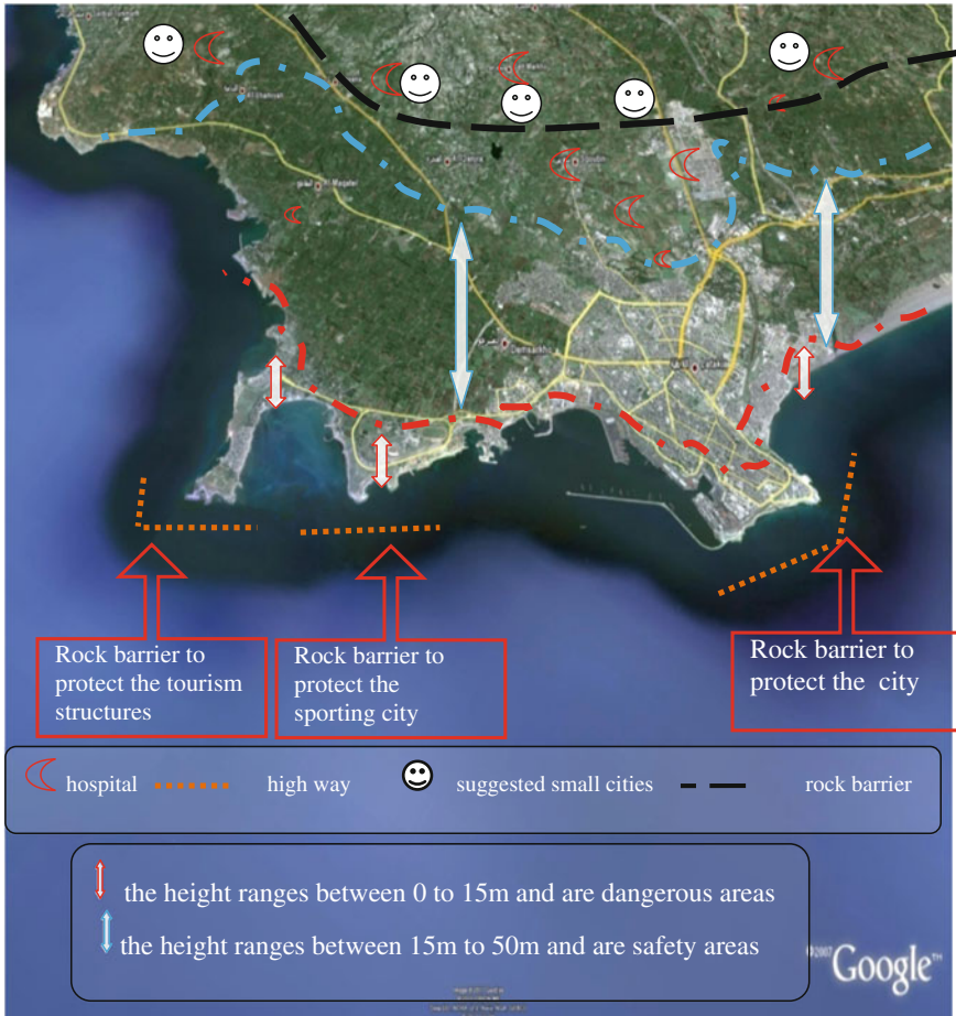
Fig. 24.24 The proposed high rock barriers against SLR on the coast of Lattakia
