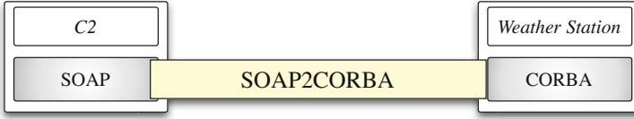
Fig. 6. Pairwise mediation between layered protocols
