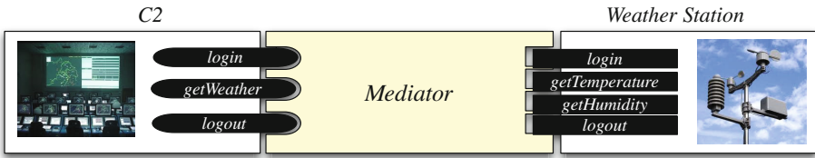
Fig. 5. Mediator to solve architectural mismatch between C2 and Weather Station
