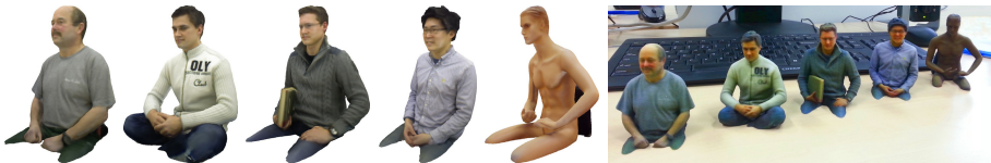
Fig. 5. More examples of 3D models acquired with our approach and the resulting printed figures
