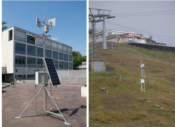
Fig. 2. Initial and final installation setup of a wireless mesh node for support to environmental research.
