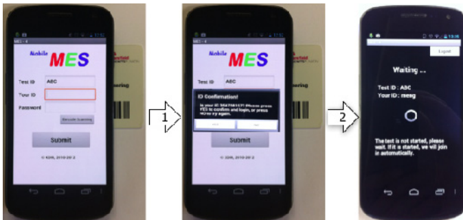
Fig. 7. Work flow of NFC recognition approach
