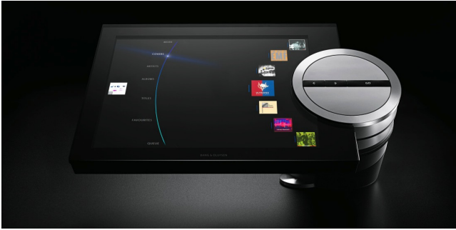
Fig. 1. Bang & Olufsen BeoSound 5. The side-mounted dial is used to scroll the on-screen content.
