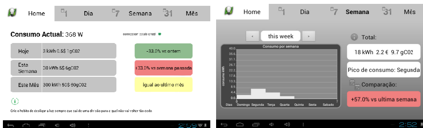
Fig. 6. Left: Home screen of the system. Right: Tab with the consumption of the current week
