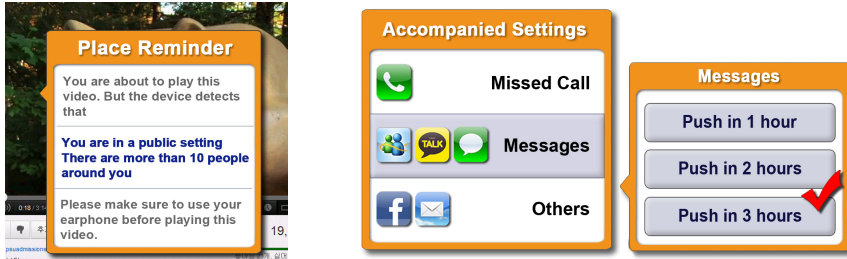
Fig. 6. Prototype of an interface that alerts users about the location and the number of people around them (left) and prototype of an interface that can be customized for pushing updates at regular intervals (right)
