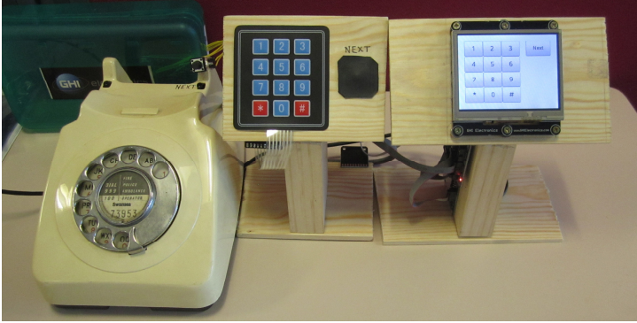
Fig. 2. The three telephone-style interfaces used by participants: the rotary dial (left), pushbutton keypad (middle) and touchscreen keypad (right)
