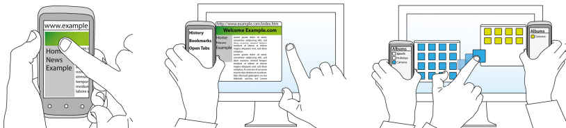
Fig. 2. (left) The mobile user interface allows for the display of a limited amount of information. (middle) Connecting the mobile and an external display extends the available screen space. (right) Items can be shared with others via drag-and-drop to another connected mobile device.
