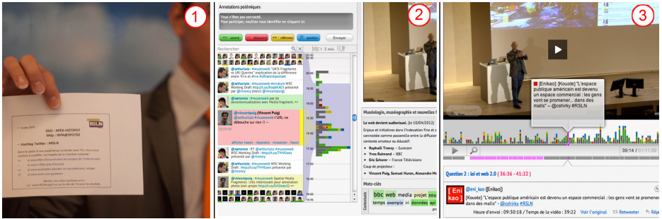
Fig. 1. The three stages of PolemicTweet: 1) printed information on connection & tags, 2) the live Twitter client & structured annotations, 3) video player showing tweet annotations
