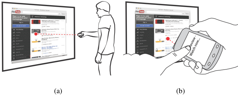
Fig. 8. Using the mobile phone as a remote control for browsing web pages on a TV set
