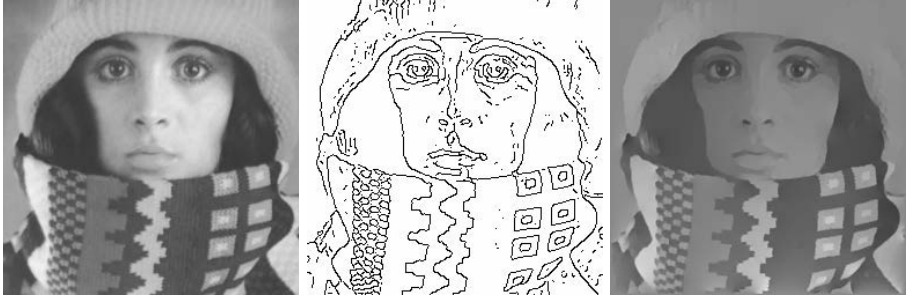
Fig. 2. Osmosis for compact image representation. (a) Left: Original image. (b) Middle: Canny edges, amounting to 9.6% of all pixels. (c) Right: Reconstruction using the average grey value of the original image and the canonical drift vectors in the edges.
