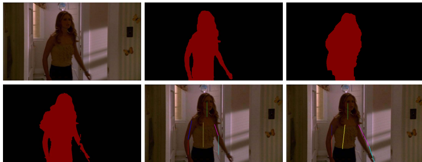
Fig. 4. Qualitative results on Buffy dataset [2]. From left to right: (first row:) input image, ground truth of segmentation, segmentation output before joint estimation, (second row:) segmentation output after joint estimation, pose output before joint estimation, and pose output after joint estimation. (Best viewed in color)
