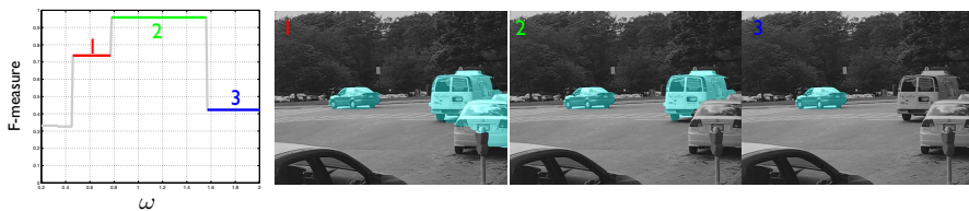
Fig. 4. F-measure scores for pixel level classification results obtained by varying \omega between 0.2 and 2. The F-measure remains constant for the intervals depicted in red, green and blue. Hence, we only show one exemplar solution from each interval.
