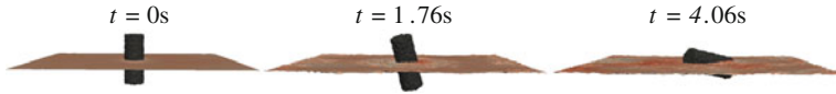
Fig. 2 Snapshots of the dynamics of a floating pile, at three different instants in time, when placed at the interface between air and water
