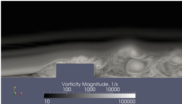
Fig. 6 Instantaneous vorticity magnitude at time t = 0.0068 s for the step with l/h = 2.7
