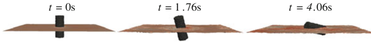
Fig. 2 Snapshots of the dynamics of a floating pile, at three different instants in time, when placed at the interface between air and water
