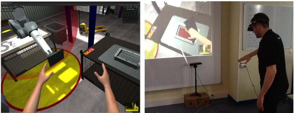
Fig. 1. Avatar’s hands trying to pick-up the part from the robot (left) and user trying to put the part in the metallic die (right)
