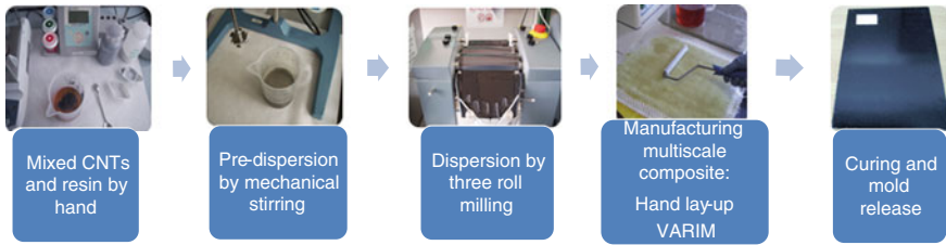
Fig. 5 Scheme of manufacturing nanocomposite
