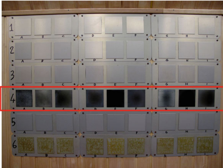
Fig. 15 Silver nanocluster/silica composite coating on aluminum alloys for space application in the MARS 500 experiment
