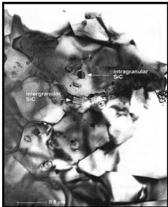
Fig. 6 Actual microstructure of a SiC-Si 3 N 4 nanocomposite [31]
