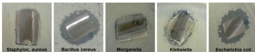
Fig. 10 Inhibition halo test against different bacteria of the silver nanocluster/silica composite coating deposited on Combitherm ® substrates
