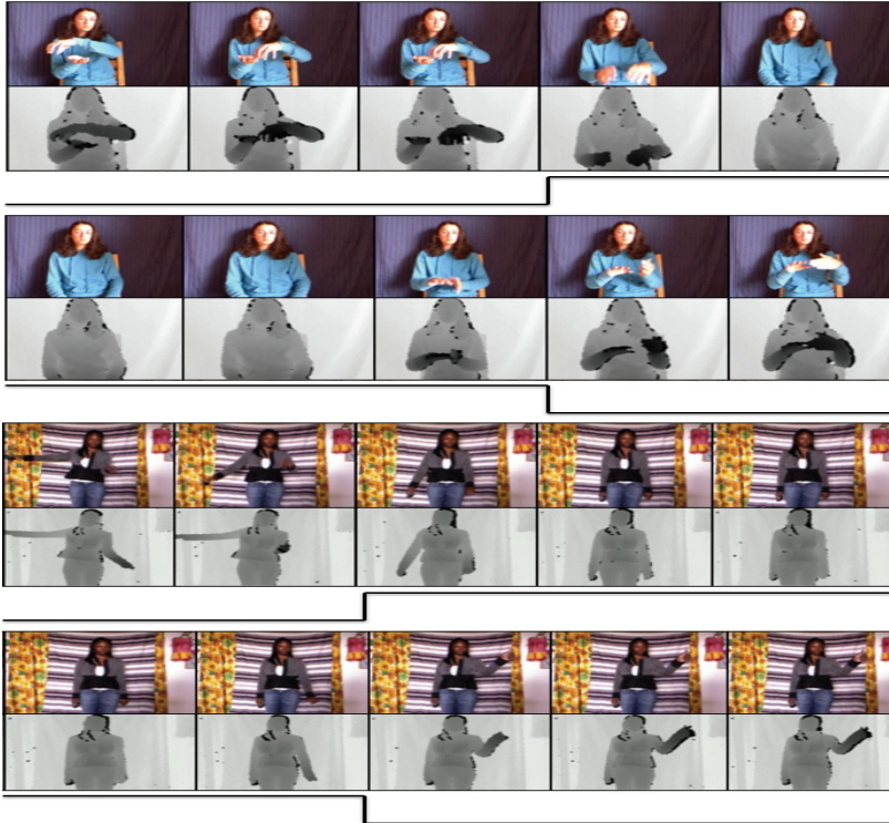
Fig. 4. Examples of resting gesture detection on the Chalearn dataset using the probability-based DTW approach. The line below each pair of depth and RGB images represents the detection of a resting gesture.
