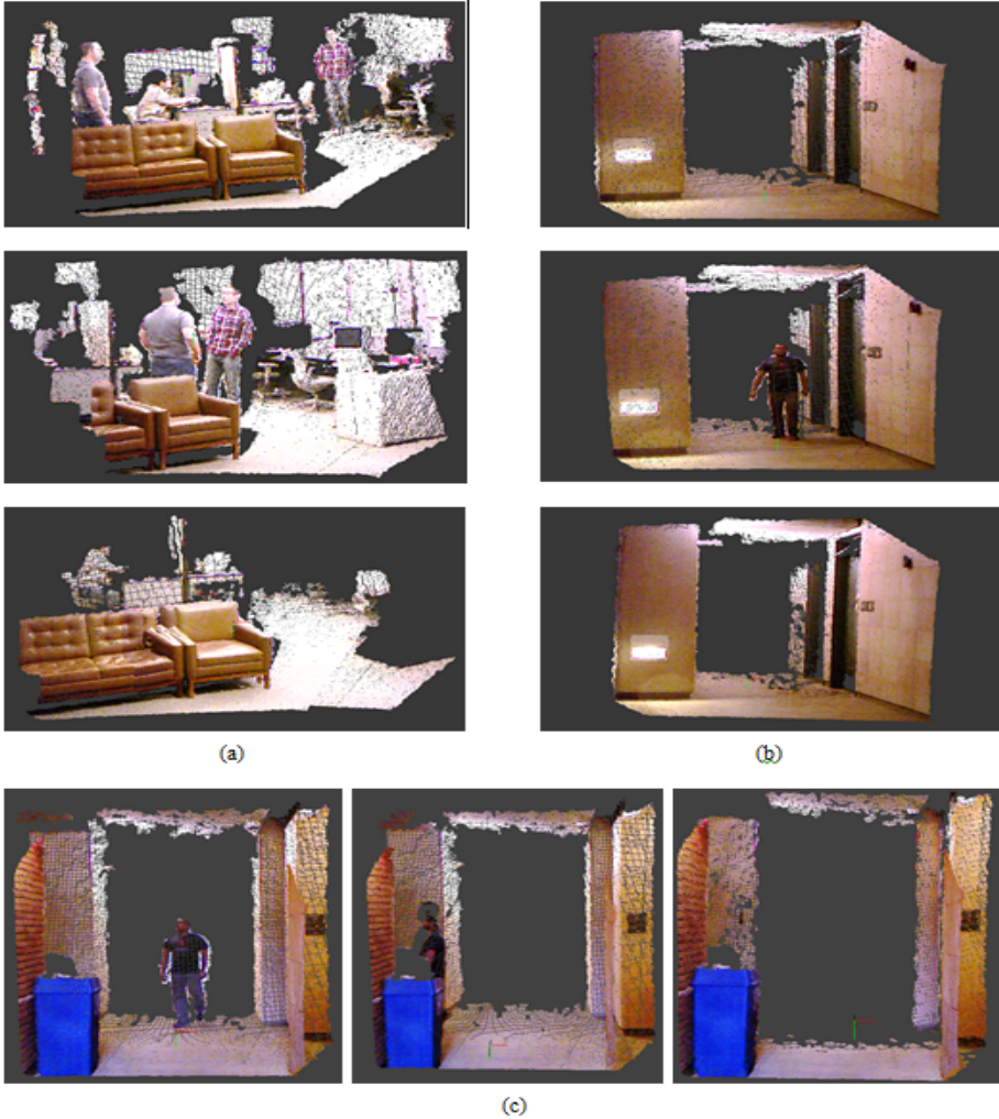
Fig. 5. Example results. (a) office scene with three people (two walking, one sitting). The top two frames from columns (a) and (b) were merged together to produce the bottom point cloud. (b) corridor scene where the person just entered the corridor through a doors on the right. (c) a walking person changing direction.
