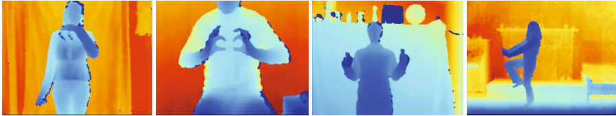
Fig. 1. Kinect TM data. Color rendering of depth images from the gesture challenge database were recorded with a Kinect TM camera. Regular RGB images are recorded simultaneously (not shown). Kinect TM can record videos with up to 30 frames per second.
