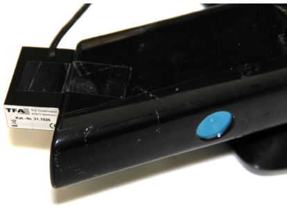
(a) Temperature sensor (left) attached to Kinect's ventilation slot.
