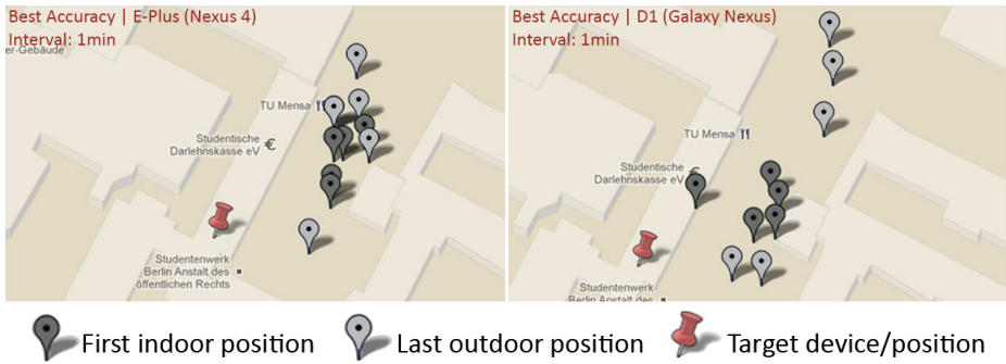
Fig. 5. Measured outdoor (light) and indoor (dark) positions for two different cellular networks (E-Plus 1800 MHz and Deutsche Telekom D1 900 MHz)
