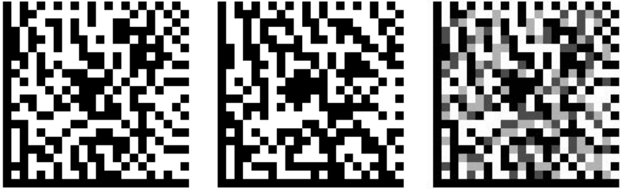
(a) Data-Matrix Layer 1: \mathcal{E}_m(s) (b) Data-Matrix Layer 2: \mathcal{E}_m(t) (c) Dual Data-Matrix Code E_d(s, t) with \alpha = 0.7
