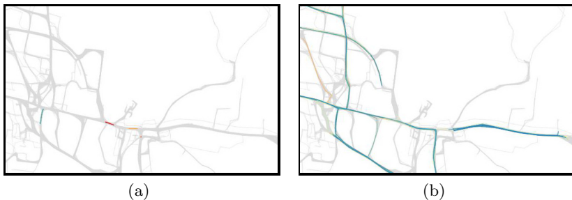
Fig. 6. (a) Trajectory Clusters of the Trucks Discovered by Traclus and (b) Frequent Routes of the Trucks Discovered by Algorithm A-1 in the Same Area
