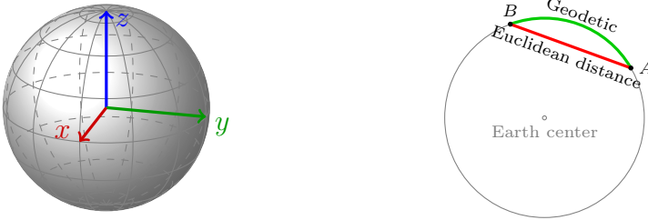
(a) ECEF coordinate system: x is to 0^\circ N, 0^\circ E , y is to 0^\circ N, 90^\circ E , z to 90^\circ N (b) Euclidean distance is a lower bound for geodetic (great-circle) distance
