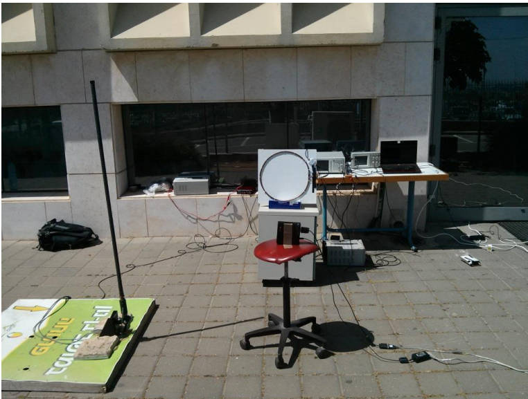
Fig. 7. The full range extension setup outside our building. The victim reader is located on the lab stool in the middle of the picture. The uplink antenna on its ground plane is on the left. The downlink loop antenna is behind the reader. The victim tag is on the table in the back, next to the laptop running the relay software.
