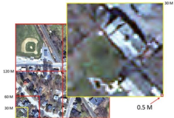
Fig. 2 An example of the raw 0.5 m orthoimagery, and the 120 m resolution cells it is aggregated to
