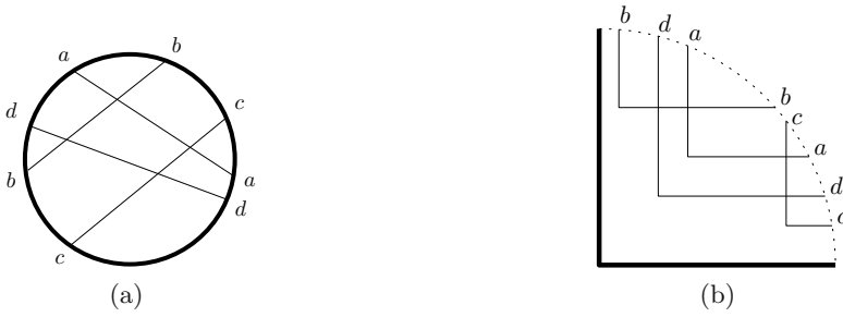
Fig. 2. (a) A circle diagram. (b) Each chord is replaced by a single-bend path on the grid.
