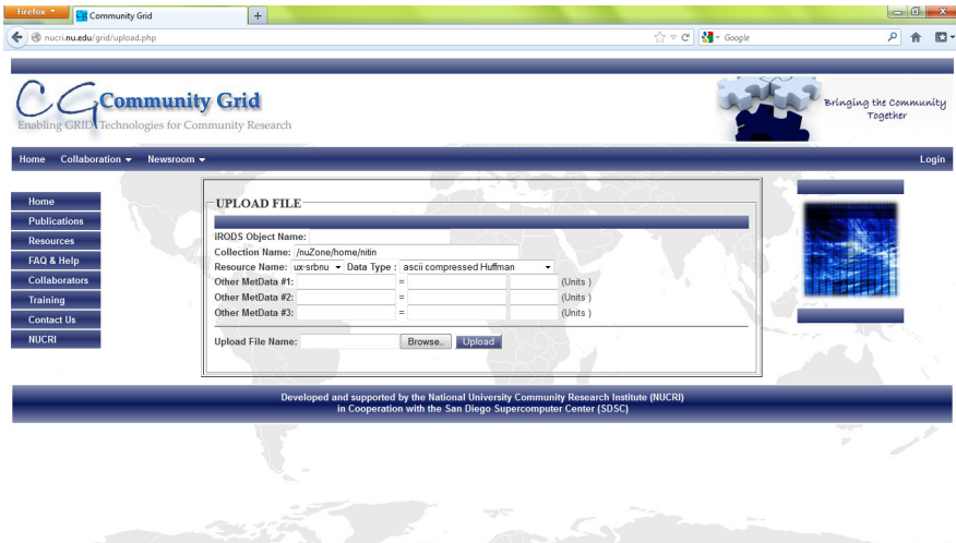
Fig. 3. Web-based portal interface for uploading the files in the C-Grid. An upload file web page is for users to upload and to copy a local file into the data grid. The fields such as, iRODS Objects Name, Collection Name, Resource Name, Data Type and Upload File name are necessary for successful uploading action and metadata creation.
