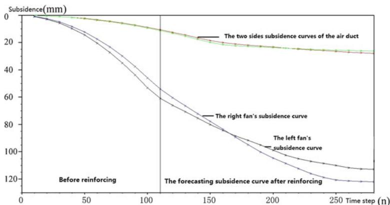
**Fig. 7** Curves of return air duct subsidence simulation
