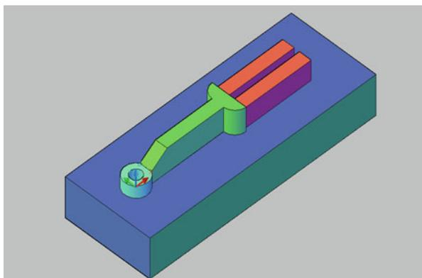
**Fig. 1** The 3D model of the return air duct
