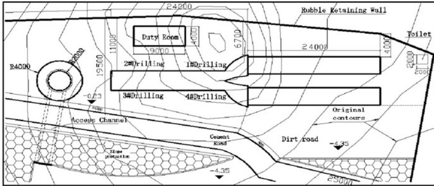
Fig. 4 Schematic diagram of drilling hole layout and the original terrain contour lines round the duct
