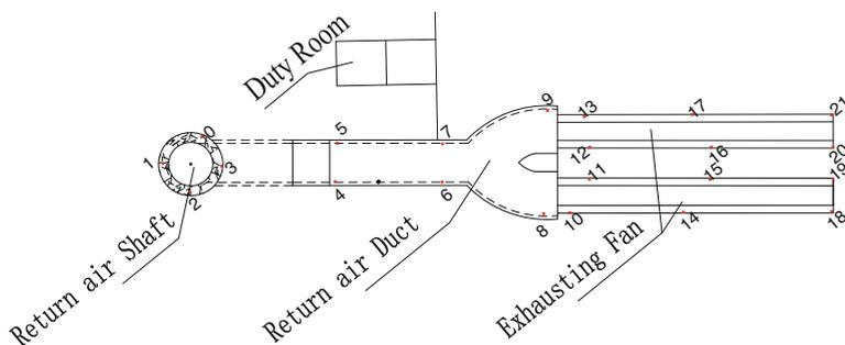
**Fig. 3** Sketch map of air duct settlement observation points layout
