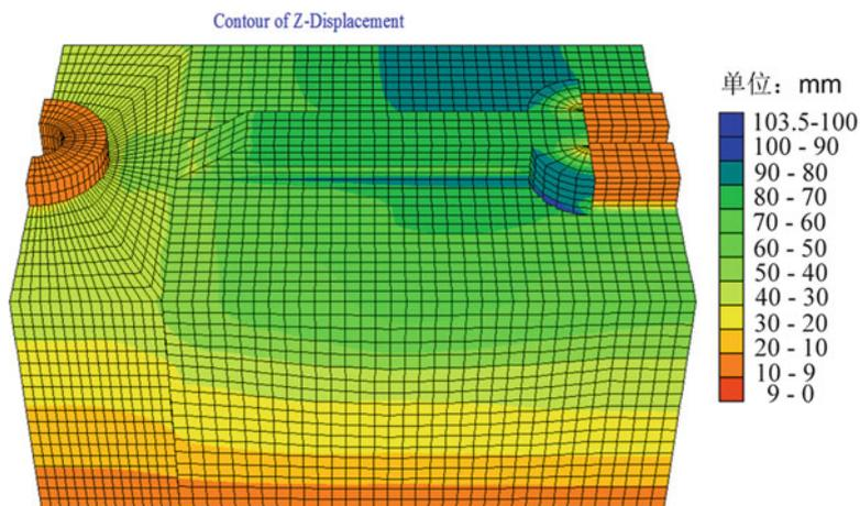
Fig. 6 Result of subsidence numerical simulation
