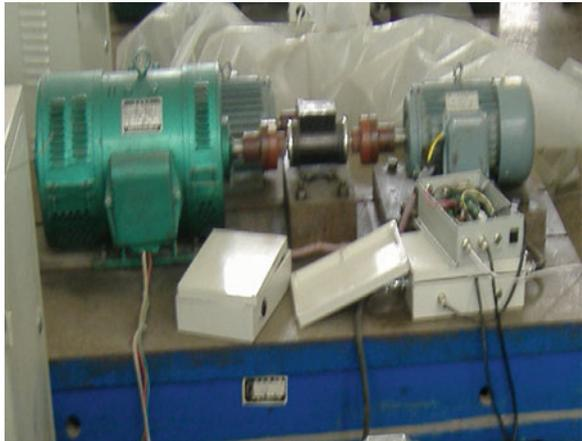
**Fig. 1** Bench of induction motor
