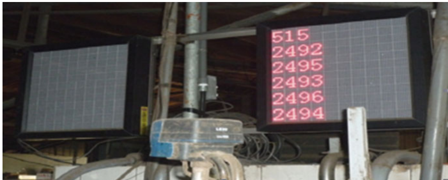
Fig. 6 The LED monitor displays the cattle ID that has been read
