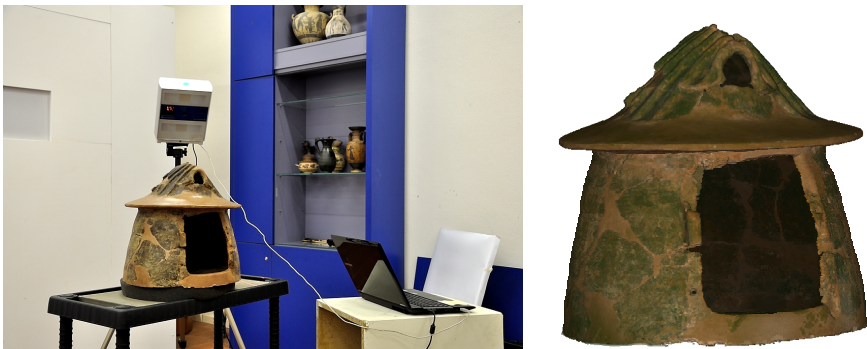
Fig. 1. 3D scanning of the Vetulonia urn at the Grosseto museum (left) and a snapshot of the 3D model of the Vetulonia urn (right)
