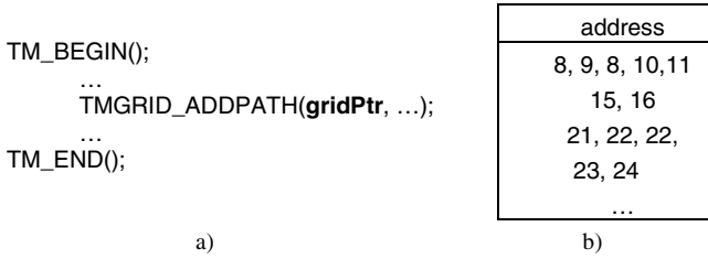
Fig. 2. a) Part of the Labyrinth program. b) Memory addresses (in granularity of cache block) pointed by gridPtr in Labyrinth.
