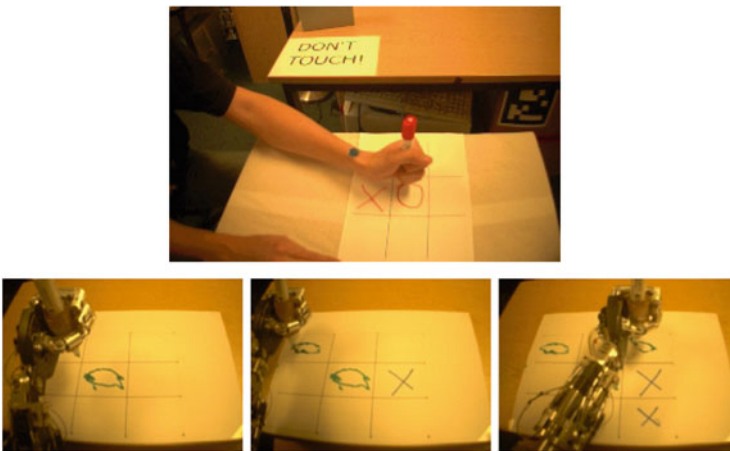
Fig. 9 Using OSILA to adapt learned templates to new board positions using the iCub humanoid in a tic-tac-toe game
