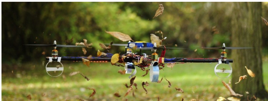
Fig. 2. Photograph of the flying NeuroCopter. The quadrotor frame is built from carbon fiber tubes and an aluminum cross joint. The flight control electronics based on the Arduino platform, motors and power supply are standard components. A Linux board is used for wireless communication, camera readout and basic computations. Most processing is done on the ground station's computer.
