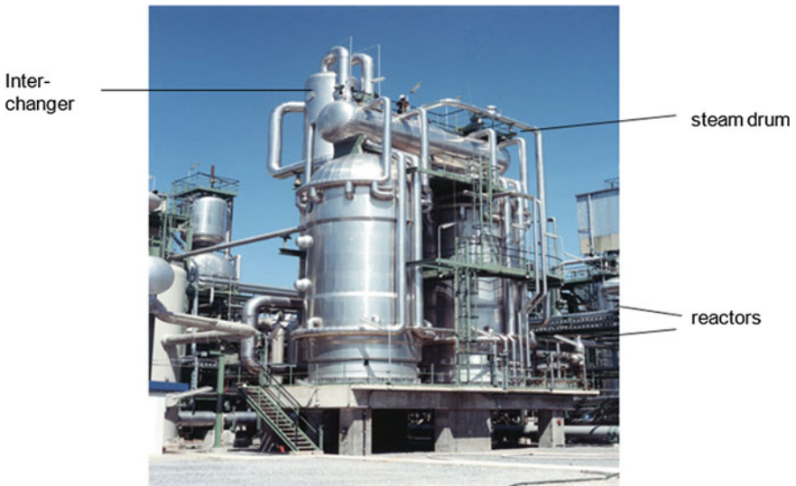
Fig. 4.111 Lurgi reactor system with two parallel water-cooled reactors. (Courtesy of Air Liquide Global E&C Solutions)
