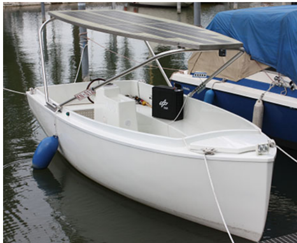
Fig. 6.126 Micro-direct methanol fuel cell of 100 W, applied as support for the solar battery system, by DLR
