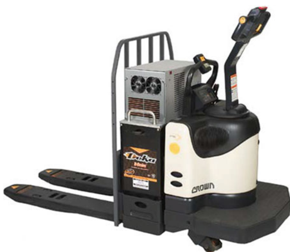
Fig. 6.127 OorjaPac direct methanol fuel cell power pack
