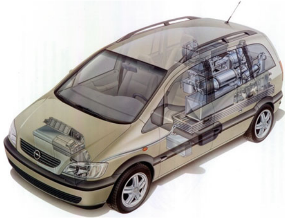
Fig. 6.139 Opel/GM-Zafira methanol concept car with reformer and fuel cell (1998)
