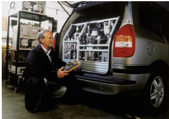
Fig. 6.140 Opel/GM-Zafira methanol concept car with reformer and fuel cell in the rear
