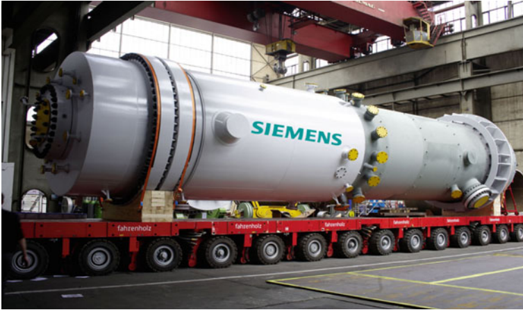
Fig. 4.61 A 500 MWth GSP gasification reactor
