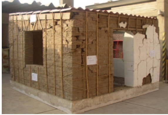
Fig. 28 External cane-rope mesh reinforcement [80]
