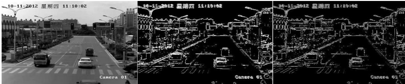
Fig. 2. The original gray image (left), LBP image (middle), the simplified LBP image (right)
