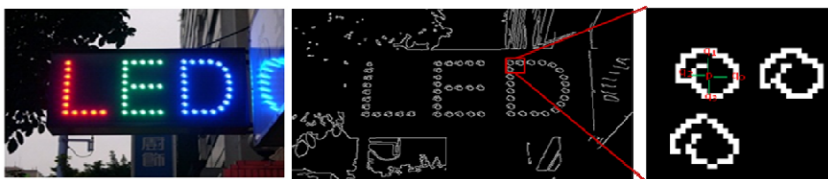
Fig. 3. The interesting point extraction. The center image is the edge image after applying canny edge detector on the left image. In the right image, the point p is the interesting point candidate, while q_0, q_1, q_2 and q_3 are associated points of p (in this case m=4 ).
