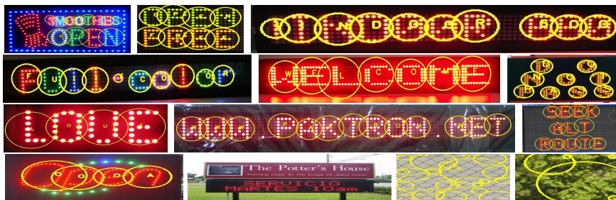
Fig. 5. Some example results of our proposed method. The results are marked with yellow circles and recognized characters. Note that the LED texts are detected in full image, but we only show cropped subimage due to space limitation. The last row shows failures of proposed method; (the first image) our method can detect the LED text, but the recognizing results are not true due to slanted text. (the second image) missing detection due to continuity of the LED text. (the remaining images) false positive due to repeating patterns.
