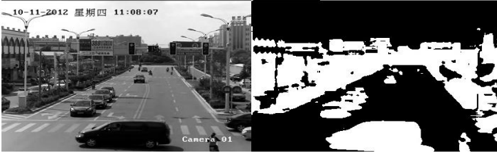
Fig. 1. Vehicle detection. The gray image (left) and its the modified local variance (right)
