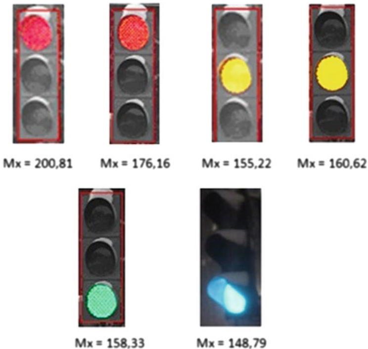
Fig. 4 Traffic light color change depending on environmental conditions
