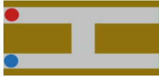
Fig. 1 Two groups of occupants (denoted by the blue and red spheres ; walls are shown in brown ) in a simple scenario with high symmetry: the exits (shown in green at the right side ) are equally far away and have equal capacity. If the two groups have equal size in number and the occupants of both groups have comparable walking speeds it would not make sense to use the connecting corridor as it would imply a time delay
