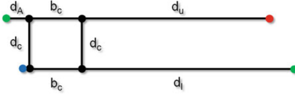
Fig. 4 Simplified network display for the paper and pencil calculation. The lengths of the links are d_A = 4 m, b_c = 5 m, d_u = 38 m, d_c = 5 m, d_l = 43 m
