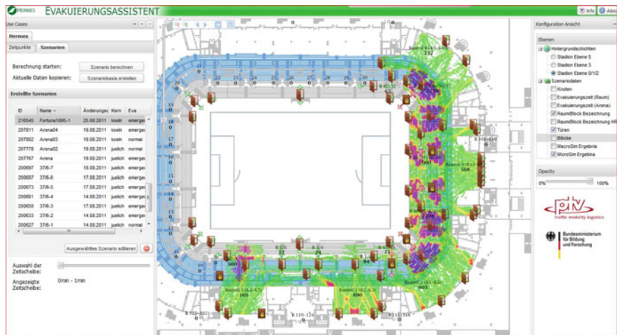
Fig. 2 The evacuation assistant showing the results of a simulation. The congestion areas are displayed
