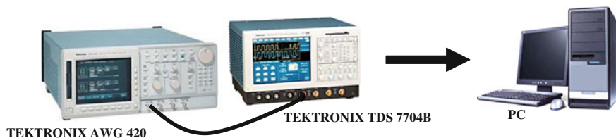
Fig. 13.8 WER measurement setup
