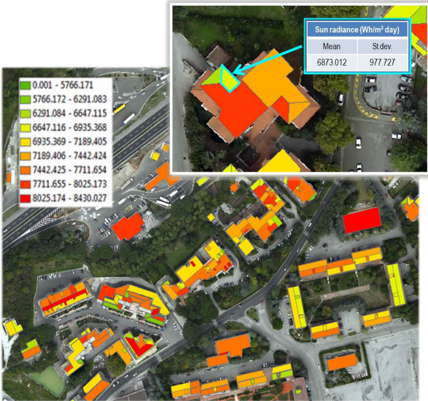
Fig. 10. Detailed map of subarea included in Figure 9 (red box) with the daily (July) cumulated sun specific radiance indication (values in Wh/m 2 day) for each roof surface extracted from DSM and characterized as GIS polygonal data. Aerial true-color orthophoto on background
