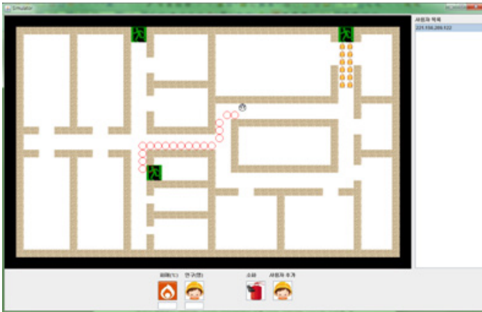
Fig. 4. Simulator for Fire Escape Support Service
