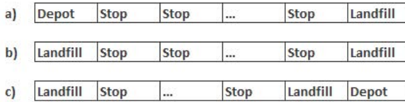
Fig. 2. Three types of a sub-route in waste collecting vehicle routing problem
