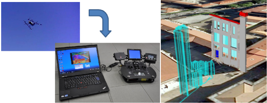
Fig. 6. Thermal signal recording system (left) and UAV path in blue (right)
