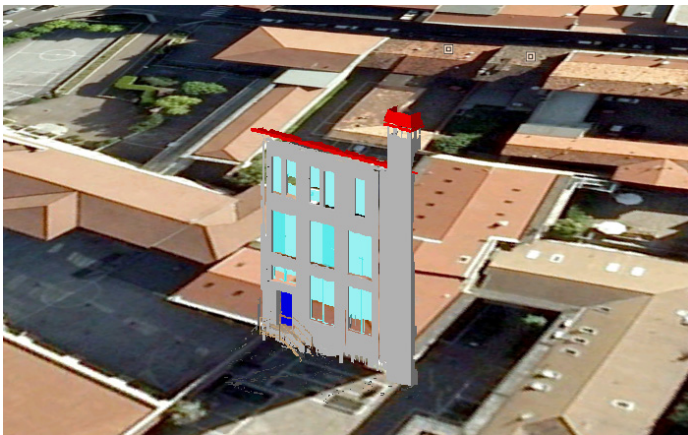
Fig. 9. The CityGML façade model enriched with semantic information on a orthophoto
