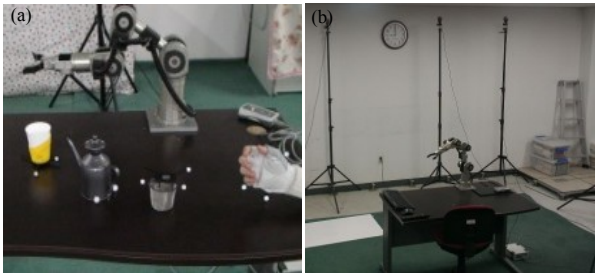
Fig. 3. Illustrations of a robot arm and a motion capture system: (a) Katana robot arm and four objects (i.e., cup, kettle, teabag, and human hand) and (b) Experimental environment containing a robot arm and a motion capture system
