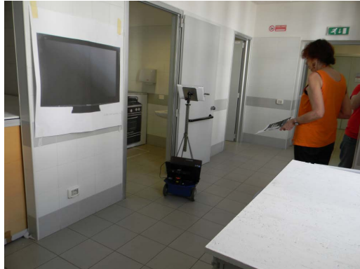
Fig. 3. A user attending our usability study meanwhile controlling an Erratic robot within a home environment through our voice interface
