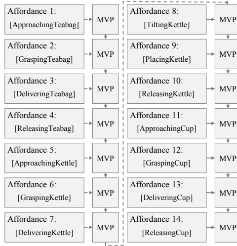
Fig. 5. Motivation graph for executing tea service task. Here, fourteen affordances are used for achieving the task.
