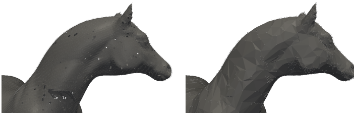
Fig. 2. Mesh reconstruction and optimization from 93836 to 20795 triangles
