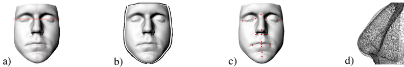
Fig. 1. Face elastic registration: a) origin point, b) detection of the edges curves, c) detected points, d) surface triangle grids: of elastic ( black ) and finishing registration ( light gray )
