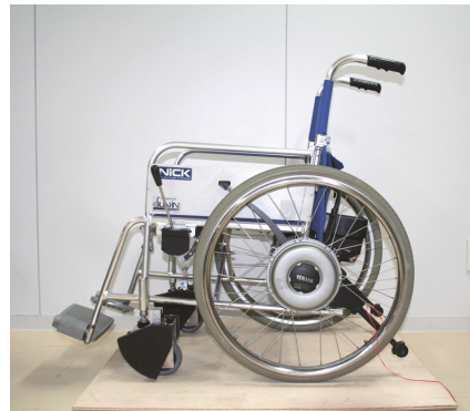
Fig. 7. Wheelchair with caster unit
