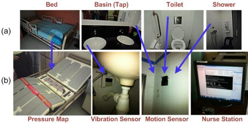
Fig. 2. Deployment of sensors and devices in nursing home
