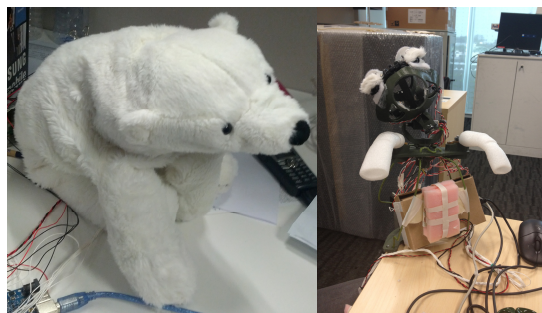
Fig. 1. Actual appearance (left) and internal structure (right) of CuDDler version 1.0
