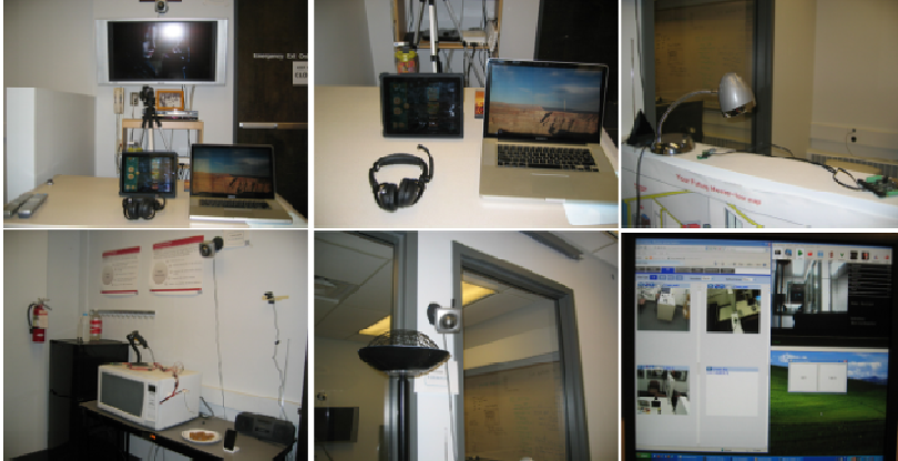
Fig. 2. Setup of experimentation in SHL. Turning on the lamp was used to synchronize the starting point when the study was started.
