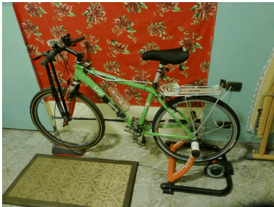
Fig. 5. Left: stationary bicycle with contact that closes and opens at every wheel rotation. Right: display showing average daily activity for the month of November 2012.
