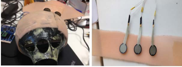
Fig. 2. Overview of a tactile sensors and interface in the Robot's head
