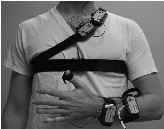
Fig. 2. Bionomadix sensor suite consisting of 3-lead ECG, respiration strap, EDA and PPG attached to the fingers of the non-dominant hand, as well as EMG sensors on the trapezius
