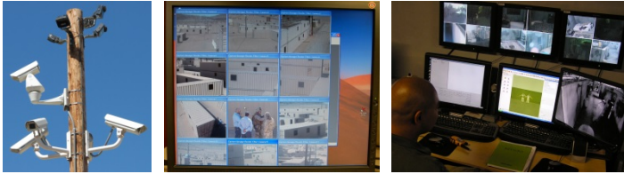
Fig. 1. A segment of a camera system with one PTZ and three fixed cameras ( left ), one screen with video feeds from 12 cameras ( middle ), and a control room with an operator ( right )
