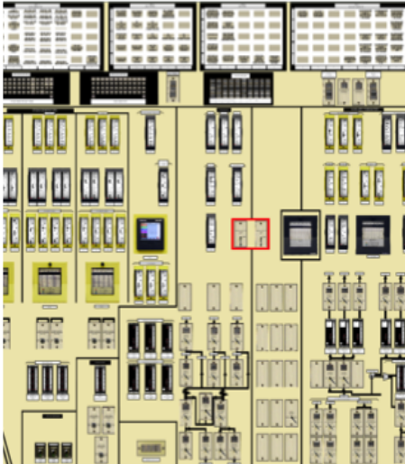
Fig. 2a. Original control panel used by operators Fig. 2b. Simplified control panel for novice participants
