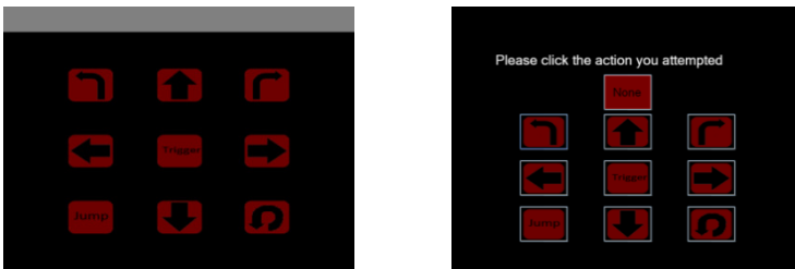
Fig. 2. Left: The 3x3 P300 BCI matrix used in this study. Right: Keyboard shown to the subject.
