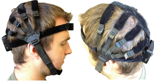
Fig. 3. Cognionics 32-channel dry EEG headset. The headset is made from soft fabric and completely encloses the wiring for the headset. The miniaturized electronics (box at the back of the head) operates from a single AAA battery and contains onboard amplification, digitization and wireless telemetry. Total system weight is only 140 g.
