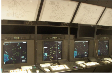
Fig. 5. ATC simulation center: Each workstation consisted of a high-resolution (2048 x 2048), radarscope, keyboard, trackball and direct access keypad
