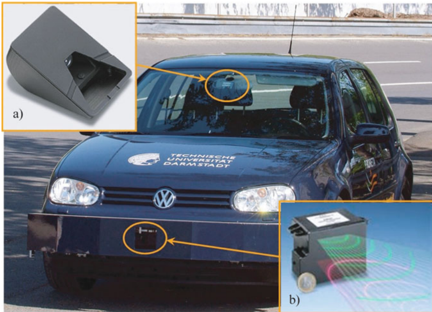
Fig. 21.3 Environmental sensors of the test vehicle: a video camera, resolution 0.07^\circ , 44^\circ , 640 \times 496 pixels, cycle time 40 ms; b laser scanner, 22.5^\circ , resolution 1.5^\circ , cycle time 90 ms
